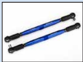
Art.Nr.: TRX7748X Vorspurstange 7075-T6 Aluminium blau 157mm (2)
