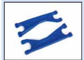
Art.Nr.: TRX7829X Heavy-Duty Querlenker blau oben 1/r v/h (2)
